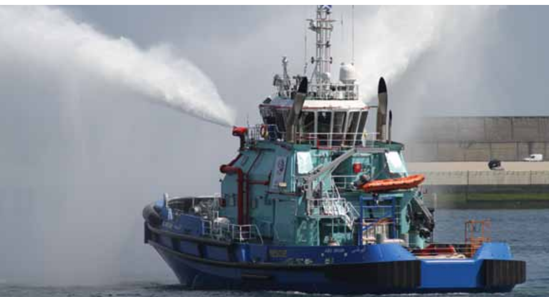
RAstar 3600 Class Alaryam testing fi-fi equipment in Abu Dhabi, UAE
